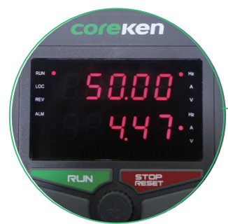
Equipped with double line digital display, compatible visual LCD optional panel design
